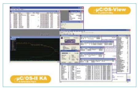
μC/OS-II is a portable, ROMable, scalable, preemptive real-time, deterministic, multitasking kernel for microprocessors, microcontrollers and DSPs. µC/OS-II can manage up to 63 application tasks and provides the following services: Semaphores. Event Flags. Mutual Exclusion Semaphores (to reduce priority inversions), Message Mailboxes, Message Queues, Task Management, Time Management, Fixed Sized Memory Block Management and more.
